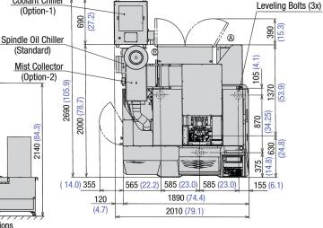
Machine Height: 90.1" Installation Footprint: 79.1" x 106.0" Machine Weight: 6,173lbs.
