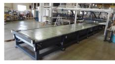
Our fully integrated conveyor options are available in either two or three sheet lengths, capacity of ½" or 1.0". Conveyors greatly facilitate lean manufacturing by allowing de-nesting in the same order as cutting.
