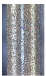
The wire EDM dress process creates a more porous surface on the wheel, allowing more grinding fluid into the cut.
