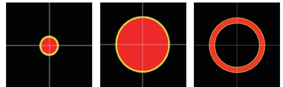
Conventional head requires three-step switching
